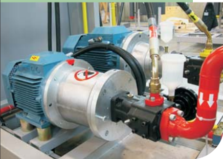
Cannon high pressure pumps with fixed & variable output can be equipped with mechanical or magnetic couplings.
