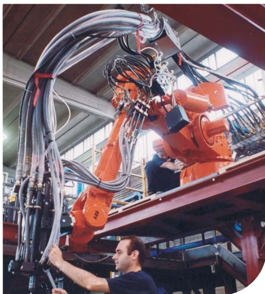
Anthropomorphic robot mounted on a mezzanine and equipped with the new Cannon FPL 32 high output head.
